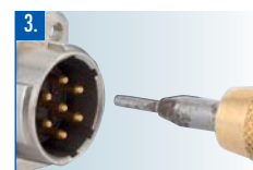
Removing the contacts
